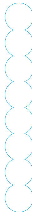
12mm x 61mm 8up flexible die Die code: M89x12v8 Order Code: V9
